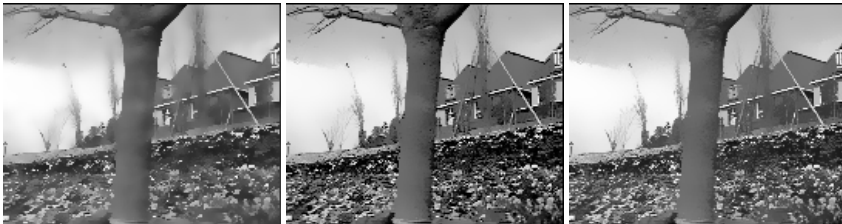
Fig. 2. Illustration of our three denoising methods with parameters p = 2 , \lambda = 0 and h = 30 after ten iterations. (a) original image; (b) noisy image; from left to right: local, nonlocal and optimized nonlocal results.
