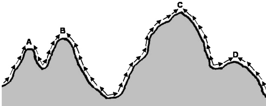
Figure 8: Possible fitness landscape for a problem with only one variable. Horizontal axis represents gene's value, vertical axis represents fitness.
