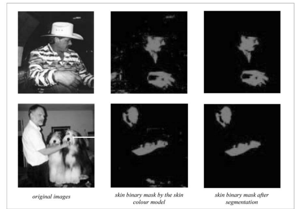
Fig. 4. Color images (left), skin pixels classification (middle), and skin regions after segmentation (right).
