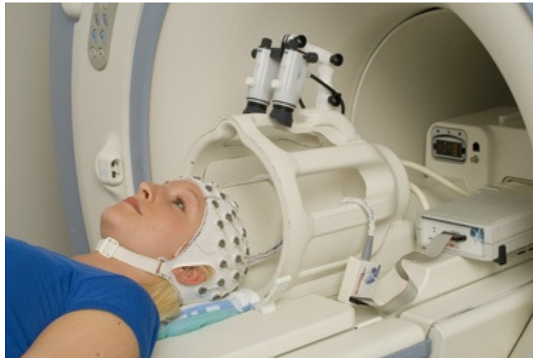
The figure shows the EEG electrode placement on the scalp when the subject is placed in the MRI head coil. From Bergen fMRI Group, GE 3.T Signa MR scanner with NNL Inc. LED goggles, and BrainProducts EEG amplifiers.
